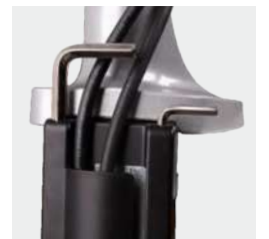
Added slots for holding tools in case of possible maintenance in future.
